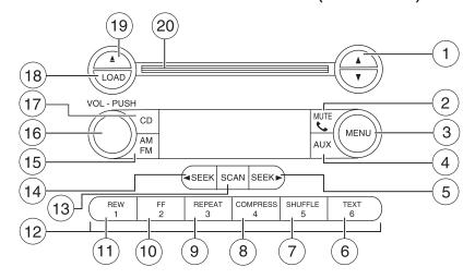
1. **A** / **Tuner:** Press to manually go up or down the radio frequency. Also use in menu mode to select various settings.
